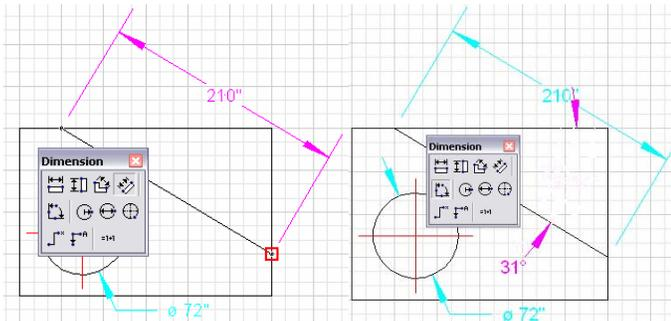
Place an Angular Dimension by selecting it from the toolbar and clicking on the lines. Click once more to place the measurement.
