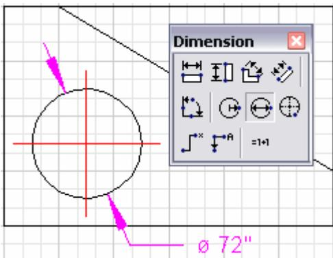
Place a Diameter Dimension by selecting Diameter on the toolbar and clicking anywhere on the curve. For a radius, do the same except select Radius.
