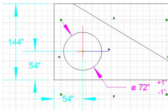
This allows for tolerancing, here +/-1. This allows for a different Label with any character on the Character Map via the Ctrl+V key combo.
